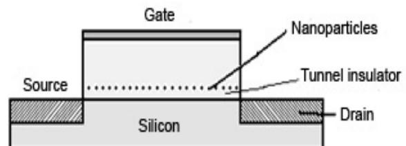
**Fig. 2. The circuit in transistors with nanoparticles**
