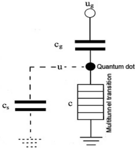
Fig. 3. Schematic diagram of single-electron memory cell
